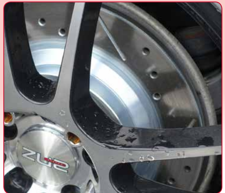
Above and below: the slotted and drilled rotors. Note that they are plated on the non-braking surface ... no nasty rusty hub!
